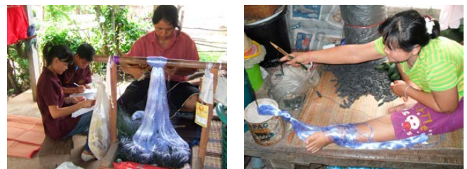
Figure 1 The main processes of fishnet home based production are lead attachment process (left) and float attachment process (right).
