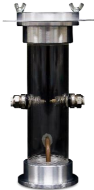
Figure 2: 1.2 L Chamber equipped with two spark plugs.
