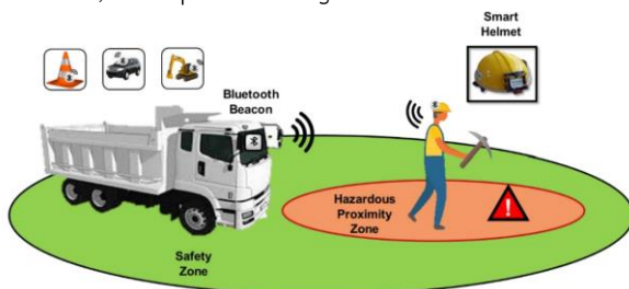
Figure 6. Overview of dangerous situations when using smart helmet 14 .
